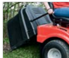
All tractors with rear discharge have a grass catcher which is easy to empty from the driver's seat.
