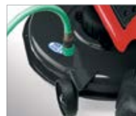
Some lawn tractors by MTD are equipped with a deck wash nozzle for easy cleaning of the deck. Note: optional on some tractors.
