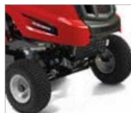
Pivoting front axle for an even and professional cut even over bumpy terrain.
