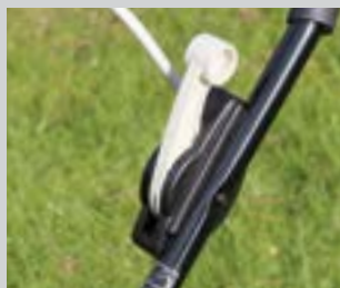
Blade engagement with safety operation control system
