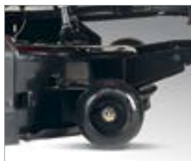
Mowing deck with antiscalp wheels to prevent damage to the grass surface.
