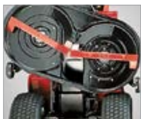
Tractors with rear discharge and a two-blade system have counter-rotating blades which transport the clippings very effectively into the grass catcher.
